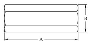
IFP Air Bleed Valves are used to remove trapped air in a hydraulic circuit or facilitate pump priming at start up when operating in a closed circuit. Unit operates by allowing air to pass at low pressure (start up) to the tank and oil flow will be closed as pressure increases.
