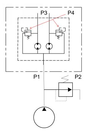
P1 = Pressure at the inlet of the Flow divider
