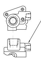
THIS TANK BYPASS CONN. IS REQUIRED FOR INSTALLATIONS WHICH OPERATE AT PUMP RELIEF VALVE PRESSURES FOR PERIODS EXCEEDING 15 SECONDS. CONNECTION MUST BE MADE BELOW OIL LEVEL IN RESERVOIR.
